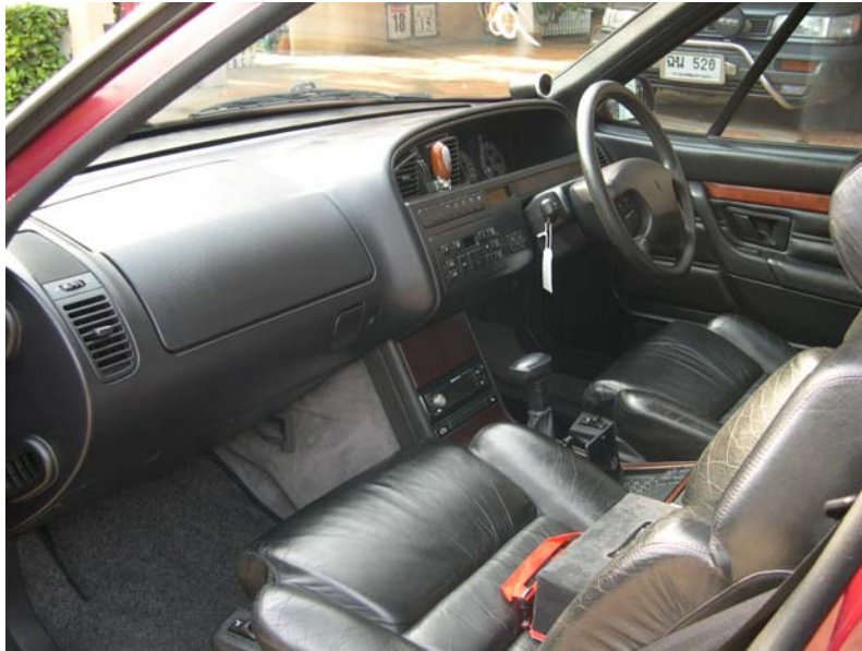
Dash Board: Airbag / Digital Climate Control / LCD warning Display
